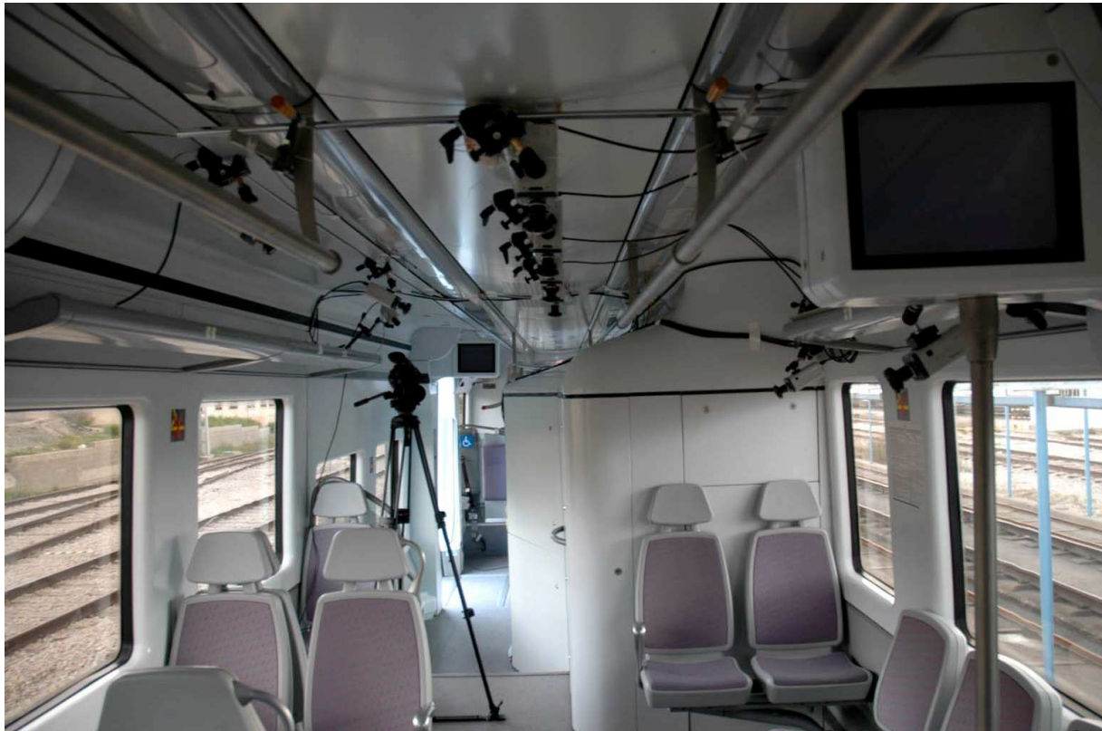
Figure 5: Sight of the cameras during the shooting (the camera on a tripod is not used for the available sequences)
